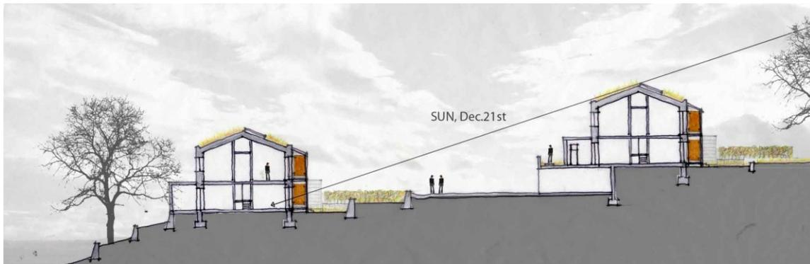
**Figure 4: The planning considers the optimal use of solar power (even in wintertime)**
